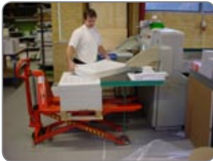
1,500 kg can be transported and lifted up to 400 mm. From 400 mm the lifting capacity is 1,000 kg.
